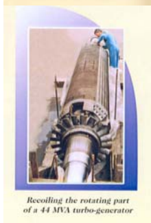
Recoiling of a 176.5 MW turbo-generator
